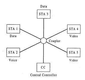
Figure 1. The network architecture in FO-CDMA
